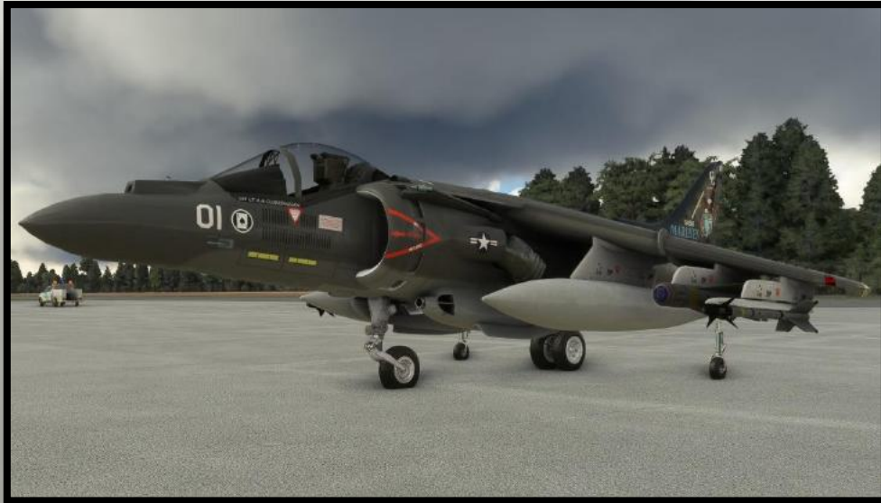
The AV-8B Plus Harrier II, with extending radar housing in the nose and FLIR sensor atop.
