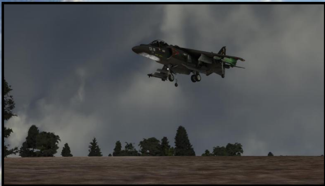
AV-8B + Harrier II demonstrates a rough-field VTOL landing – a unique capability for a fighter aircraft
